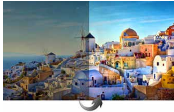
Fig. 5: Resistive touch (75%) vs. projected capacitive (93%) transmittance. The higher the transmittance level of the cover glass, the clearer and brighter the picture becomes.
