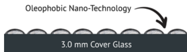
Fig. 7: The oleophobic nano-technology repels fingerprints for better visibility as well as germs for a safer work environment. It also creates a smooth surface that makes it work well with nitrile and latex gloves without skipping.
